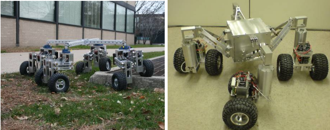
Figure 1: The IIT prototype vehicle design (left) compared to the MIT design (right)
