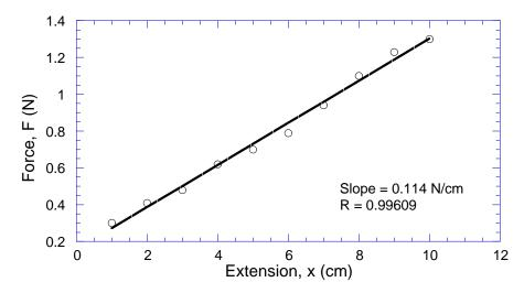
Figure 1: Experimental data of the force on a spring at various extension length (circles).
