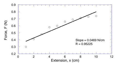
Figure 2: Another set of experimental data, but with a "bad" spring.
